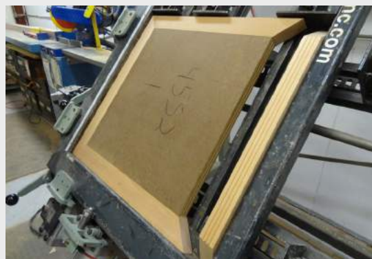
Rim Raised Panel Construction
