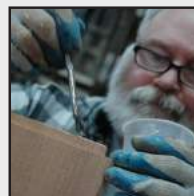
Marine epoxy is used on exterior doors; exterior grade glue is used on interior doors
